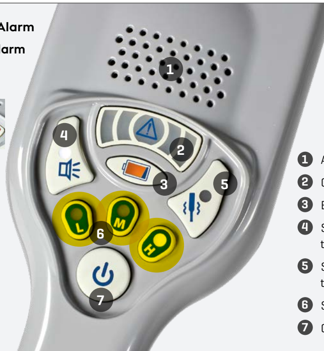
Optical indication proportional to the metal signal strength [Low, Medium, High]
